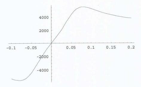
The maximum positive grip occurs, just by eyeball, around  $\sigma = 0.08$ . To the left of the maximum, adding more slip—more throttle—generates more grip. To the right of the maximum, adding more slip generates less grip. That's where we've lost traction. We can find the maximum precisely by plotting the slope of this curve, since the slope is zero right at the maximum:
