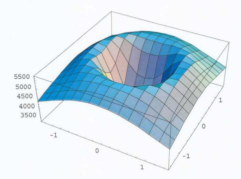
The stability criteria are visually obvious, here. If the current, commensurable slip values, s and a, are inside the central "cup" region, then increasing either component of slip increases grip. If they're outside, then increasing slip leads to decreasing grip and the driver is in the "deep kimchee" region of the plot.
