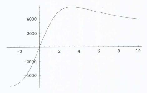
Notice the same kind of stability situation as we saw before. To the left of the maximum, more slip—more steering—means more grip. To the right of the maximum, more slip means less grip. Here's the slope:
